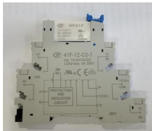
Remove from the Normally Open (NO) to Normally Closed (NC).
