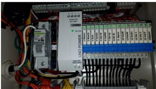
You can also open the Kleen Flo Wash Controller's lid to view the output relay's LEDs and see what output is active.
