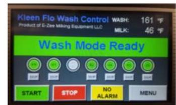
Note: The above water valves will function with the rheostat trim POTs installed. Turning the Temp up or down will determine what valve will come on for that cycle depending on the Dead Band Setting and the Temperature Fill Time Setting for that cycle.
