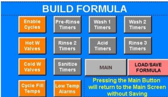
When done, press the **BUILD FORMULA** button to exit to the main *Build Formula Level 4* Menu, then press the pink **LOAD / SAVE FORMULA** button to get to the *Load / Save Current Formula* Screen.
