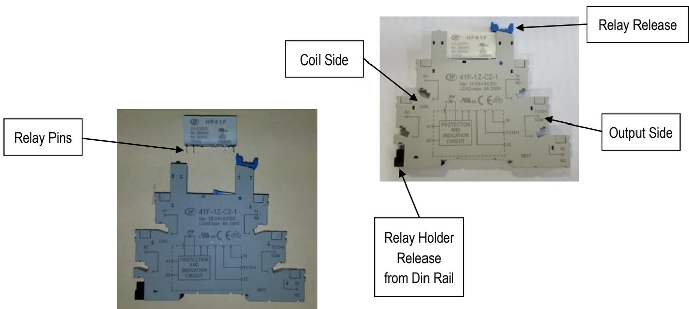
Make sure the relay contact pins are not bent and line up properly with the relay holder sockets.
