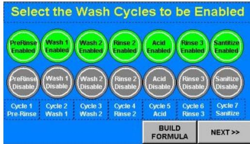
Press to make the button turn green for enabled or turn red for disabled. Select only the cycles you wish to build for that formula.
