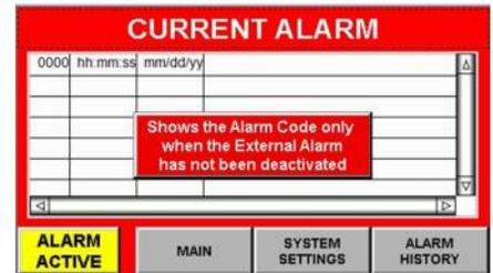
Touching the **ACTIVE ALARM** button will shut off the external alarm. The active alarm will disappear from the *Current Alarm* Screen, then an XXXX line will appear in the *Alarm History Window Level 4*, showing when the alarm was acknowledged.
