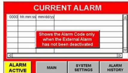
Touching the **ACTIVE ALARM** button will shut off the external alarm. The active alarm will disappear from the *Current Alarm* Screen, then an XXXX line will appear in the *Alarm History Window Level 4*, showing when the alarm was acknowledged.
