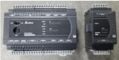
Remember to have the Stop / Run Switch in the "Run" position on the replacement CPU if replacing it.
