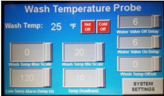
System Settings with a Wash Temp Probe
