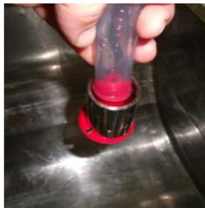
Once all wash water solution is sucked out of sink or container, you can shut off the vacuum pump and empty the bucket.
