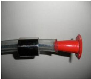
Your CIP Bucket Washer comes with 9 ft. of tubing, but you may need to shorten the length for your installation. Remove the red restrictor plug and weight, then cut tubing to desired length. Slide the weight back over the end of tubing and push the plug snugly back into place in the end of tubing.
