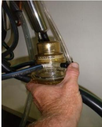
The weight of the NuPulse Goat milker, however, is not as evenly distributed. The weight of the milk hose makes the Goat milker tip down to one side and cannot wash the milker properly.
