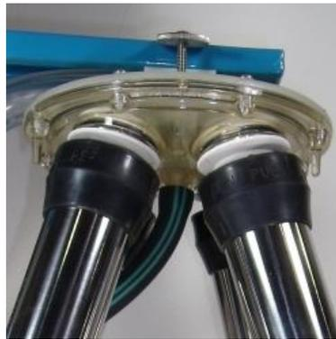
Put the NuPulse milker onto the four white jetter jets by pushing an inflation/liner onto each jet with a twisting back-and-forth motion. Next remove the black wash plug on the side of the milker and insert the adapter end of black jetter hose to that entry.
