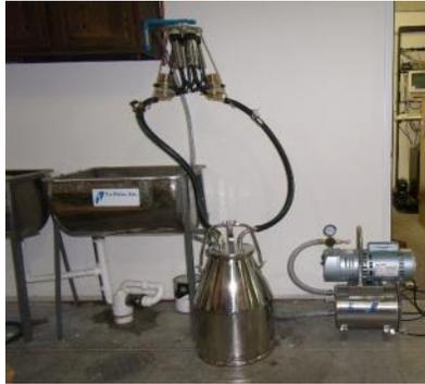
Choose your location where washing will take place. Hot water and a vacuum source are needed (i.e. portable pump). Mount CIP Unit on the wall or structure above the sink, making sure to position the CIP Unit at a height that will allow the milker(s) to reach it while on the floor (or any platform it will be sitting on, such as a wagon or cart).
